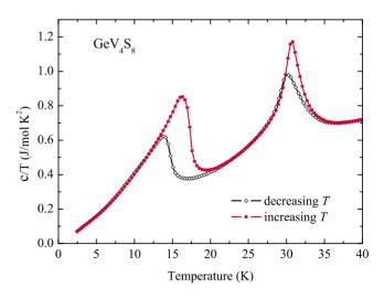
FIG. 5. (Color online) Specific heat of  $\text{GeV}_4\text{S}_8$ . Red (gray) markers: increasing temperature; black markers: decreasing temperature.
