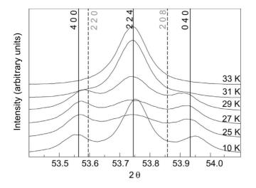
FIG. 1. Cubic (440) reflection and splitting at lower temperatures. Solid lines mark the orthorhombic reflection positions at 25 K, dashed lines mark the assumed rhombohedral reflection positions.
