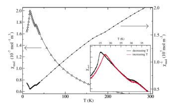
FIG. 4. (Color online) Magnetic susceptibility ( $\triangle$ ) and inverse magnetic susceptibility (+) of GeV<sub>4</sub>S<sub>8</sub> at 1 T. Insert: Hysteresis of the susceptibility measured at 0.1 T. Red (gray) line: increasing temperature; black line: decreasing temperature)
