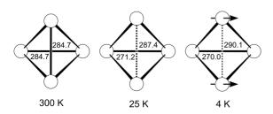
FIG. 3. V<sub>4</sub>-cluster units of GeV<sub>4</sub>S<sub>8</sub> at 300 ( $\overline{4}3m$ ), 25 (*mm*2, paramagnetic), and 4 K (*mm*2, magnetically ordered). Distances of the longest and shortest V-V bonds are in pm.
