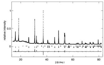
FIG. 2. Rietveld fit of  $GeV_4S_8$  at 25 K. Lower tick marks are  $GeV_4S_8$ , upper tick marks the impurity phase  $V_2O_3$
