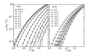
FIG. 2. Magnetic contribution to the thermal conductivity of NENP parallel to the spin chains as a function of temperature at several constant fields. The solid lines represent the calculated  $\kappa_s$  (see text). The error bars arise from the uncertainty in subtraction of  $\kappa_{\rm ph}$  from the total measured thermal conductivity.
