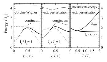
FIG. 1. One-magnon dispersion (dotted lines), band edges of the two-magnon continuum (thin solid lines), and bound singlet dispersion (thick lines) for  $J_{\parallel}/J_{\perp} = 1$  obtained from Jordan-Wigner fermions (left) and extrapolated perturbation (middle panel). Right: Energy of the Van Hove singularities of the bound singlet at  $k = \pi$  and at the dispersion maximum as a function of  $J_{\parallel}/J_{\perp}$ .
